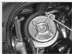
Idling speed regulating screw Standard idling speed: See page 29 (specification)
